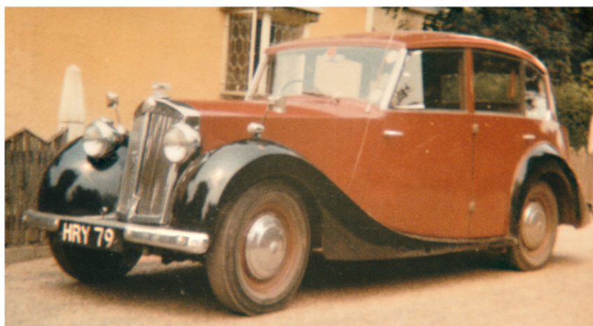
2nd car - 1952 Triumph Renown, Razor edge saloon 2L, 3 speed, aluminium body on steel chassis
